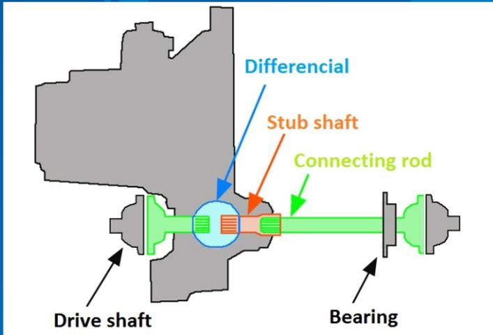
Stub shafts are a unique development of VAG which can be found mainly in Transporter and Van applications.
