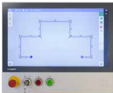
Point to Point drawing method & Real Time solution calculation during building up the workpiece design
