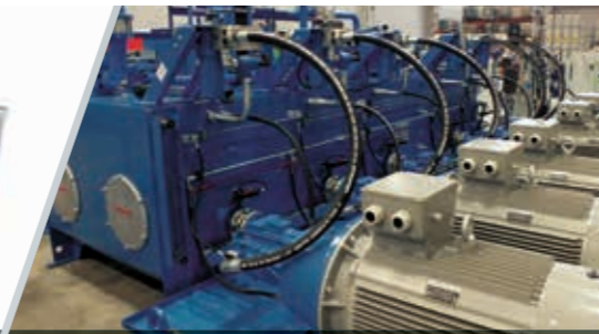
Hydraulic systems for rolling mills
