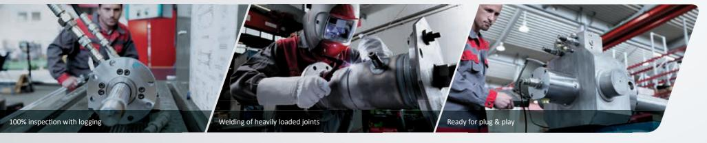
In our highly flexible production line, components for our cylinders are produced on modern machines. With the CAD/CAM link-up, smaller units can also be economically produced. In addition, our welding workshop is certified according to ISO 3834-2 and DIN 18800-7/E.
