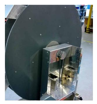
Fig. 3: The halstrup-walcher drive is located on the rear of the infusion mill
