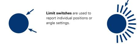
**Potentiometers** provide the current position value for every value in an angle range.
