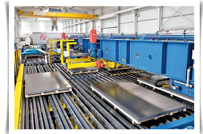
Stack packing line with magnetic belt stacker
