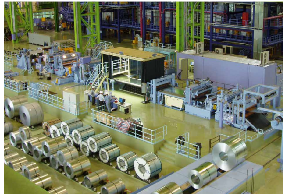
Inspection line for hot-dip galvanized cold rolled material
