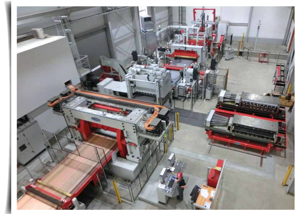
Cut-to-length line in a steel service centre
