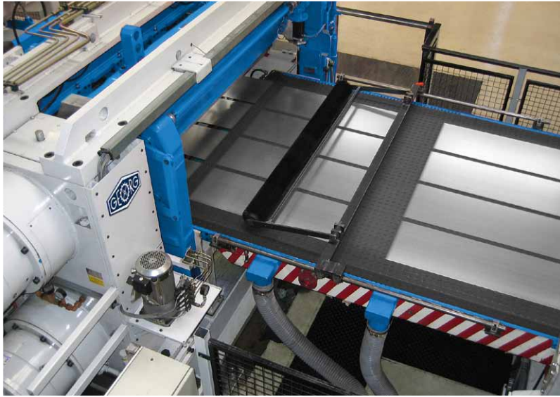
Eccentric shear for four slits in operation
