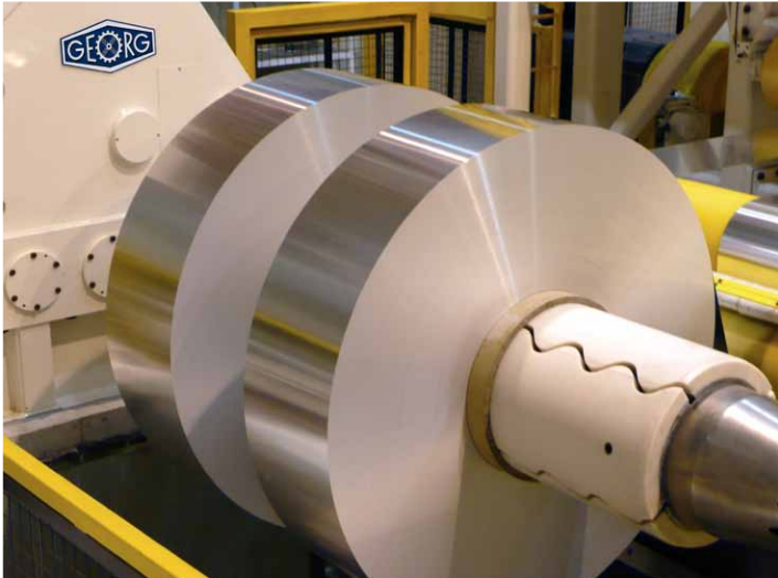
Recoiler of an aluminium slitting line
