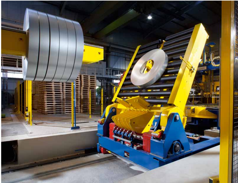
Coil separation with coil tilting table (down ender)
