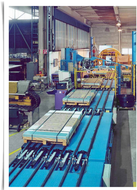
Automatic transversal strapping of the finished material
