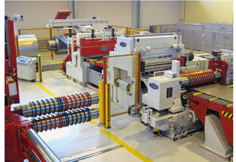
Cut-to-length line for cutting multiple strands (multiblanking line)
