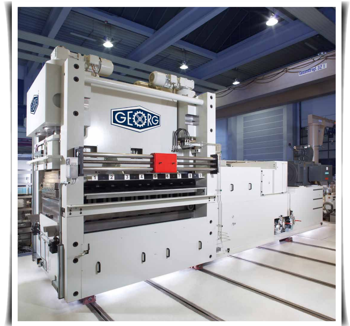
Leveller in a cut-to-length line
