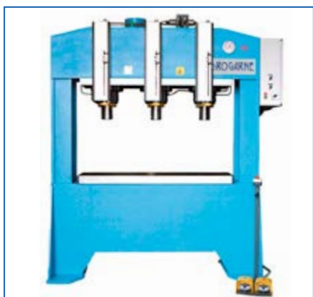
FDM-80/3 E equipped with three independent headstocks.
