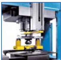
FDM-80/3 E equipped with three independent headstocks.
