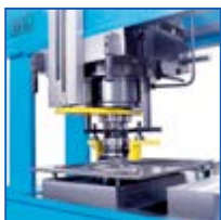
FDM-80/3 E equipped with three independent headstocks.
