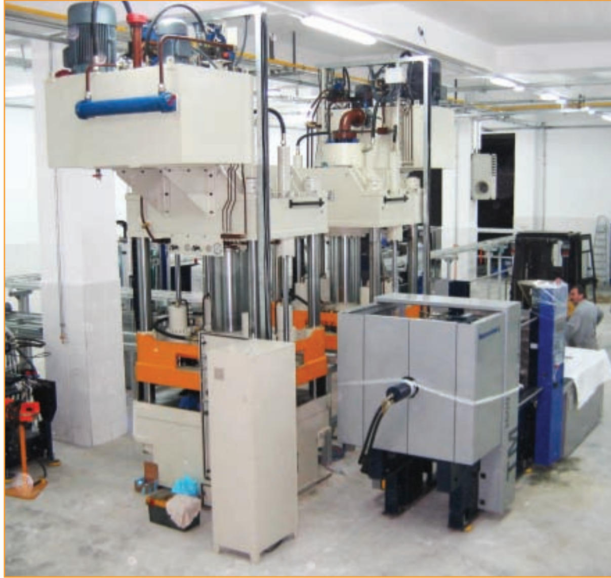
Pressan HSP 350/150 - 1260x915 Kolonlu Pres Hattı Pressan HSP 350/150 - 1260x915 Tie Rod Press Line
