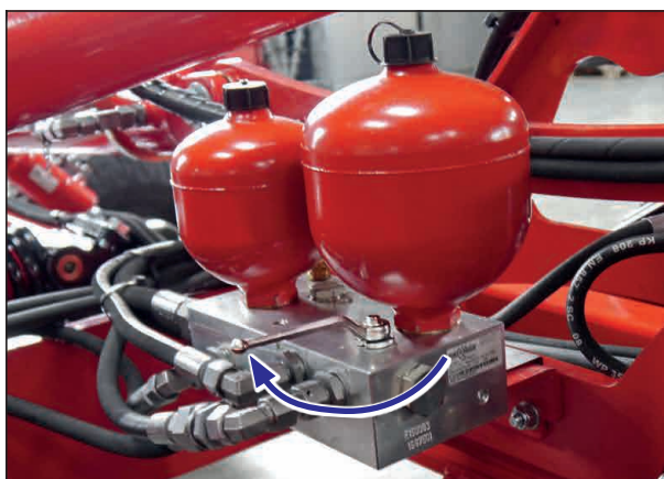
Traction intensifier lock valve - position "0"
