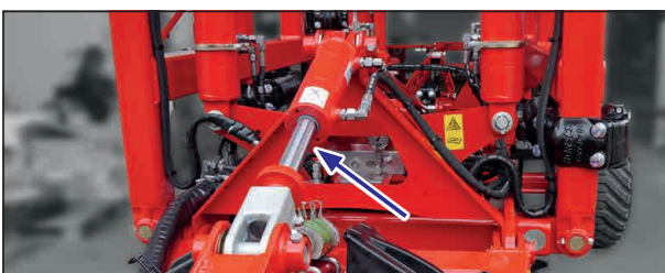
Hydraulic cylinder for drawbar
