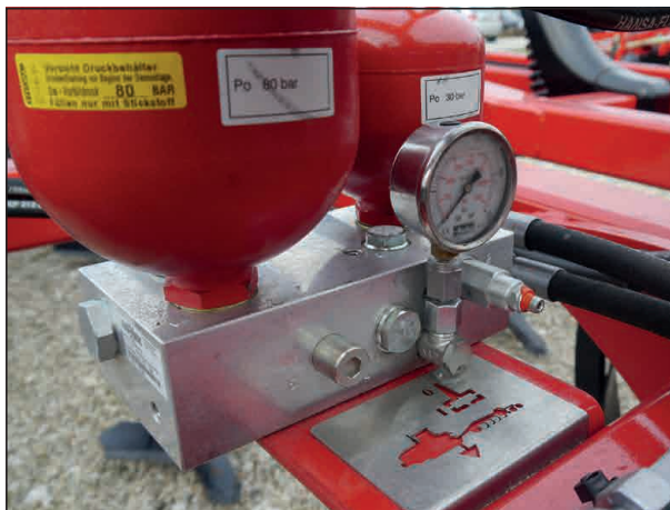
Hydraulic valve block traction intensifier with symbol plate
