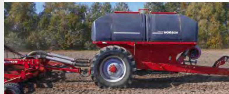
HORSCH Seed Waggon with a hopper capacity of 12 000 litre for seed and fertiliser (partition 50:50)
