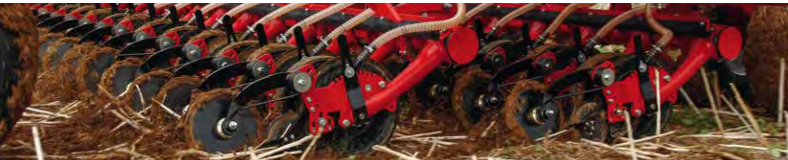
2-bar coulter design for maximum clearance
