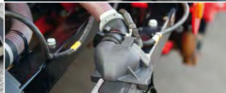
Bypass seeding system for seed rates beyond 250 grains/m 2 or seed that is not suitable for singulation
