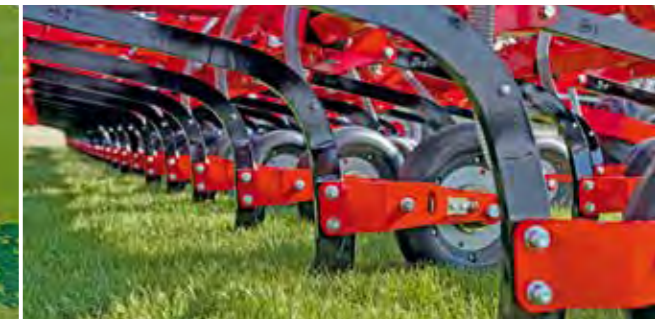
NT chisel coulters remove lumps from the seed horizon and place the grain exactly
