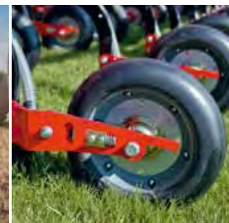
Press wheel for depth control of the seed coulters
