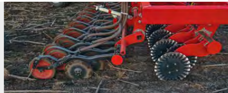
Well-proven TurboDisc seed coulters with high coulter pressure and excellent capacity to adapt to the soil for a precise seed placement
