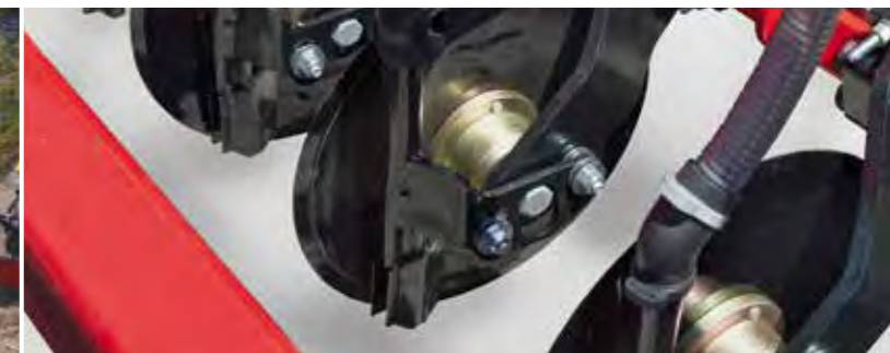
The fertiliser coulters of the HORSCH PPF system place the fertilizer at the exact depth to guarantee an optimum development of the seed grain
