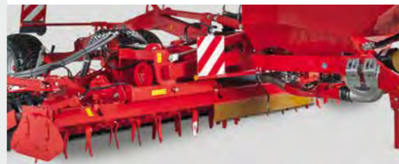
3 m segments of the rotary harrow are oscillatingly suspended for an optimum soil adjustment
