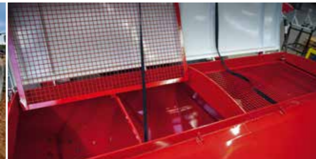
Double hopper version with the Grain & Fertiliser System (45:55)
