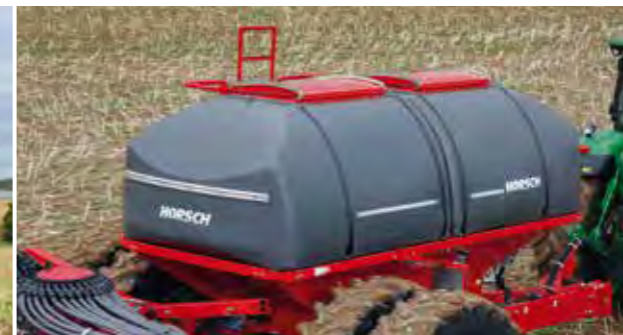
Capacity of 12 000 litre with a 50:50 split hoppers
