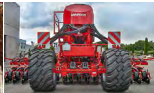
Optional: tyres 710/50 – 26.5 for maximum contact area
