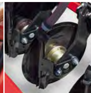
The PPF fertiliser couler is a maintenance-free double disc couler with high couler pressure
