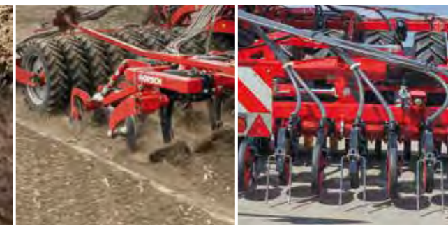
TerraGrip tines run exactly in front of the tyres
