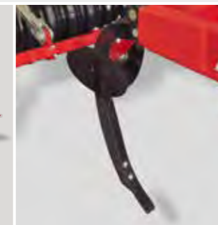
Narrow LD (low disturbance) coulters at the Terrano MT
