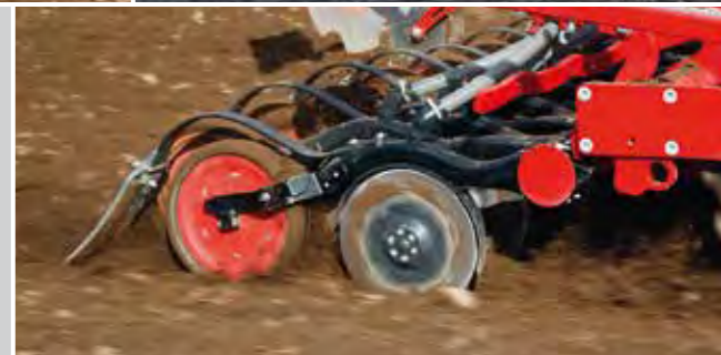
The higher than average contour following capability (15 cm) of the TurboDisc couler with integrated press wheel allows for a precise and even depth control. The high individual couler pressure of up to 120 kg guarantees smooth running at speeds of more than 12 km/h.
