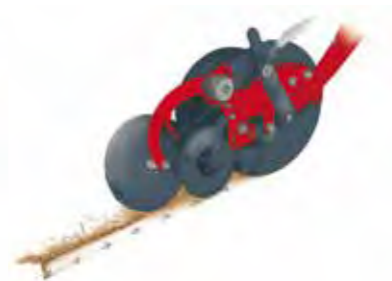
Second row Seed 2: small grains, placed shallowly, e.g. incl. slug pellets
