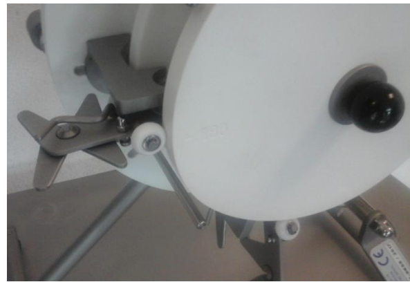
Photo 6.2. Widest point on the eccentric (indicated by horizontal mark)
