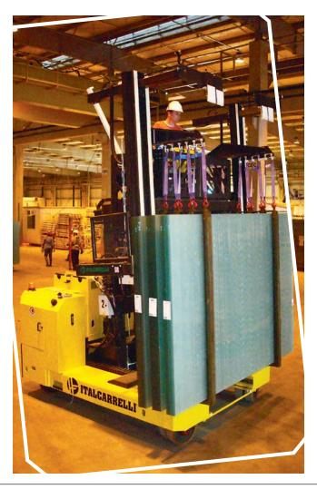
on racks - the EN4L 150C. This multi-directional sideloader can handle weights of up to 15t, and has been designed above all for our clients in Brazil, where packs of glass are mostly handled by means of special supports called collars or special racks.
