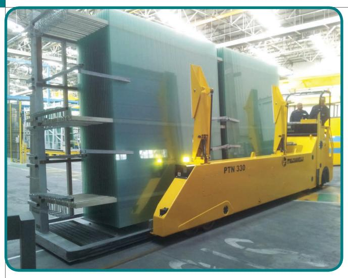
series of installations for automatic guiding, including a packaging line in a float line in Russia. This plant also includes one of our PTN330 inloaders, which have an optical guiding system that enables to automatically identify and follow a route painted on the floor. By means of this optical guiding system, the machine can also automatically and highly-precisely stop in an indicated position, ideal to place racks on automatic packaging lines, unloaders, transformation lines,
