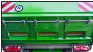
Two extra grain chutes as an option
