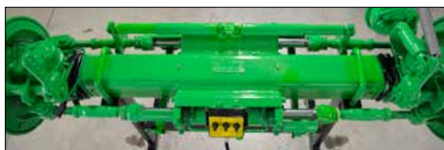
Double free steering axle
