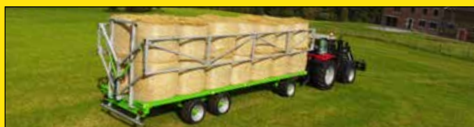
As an option on models 10000T15 and 10000T20, side hydraulic ladders (2 SA) ensure use safety and rapidity
