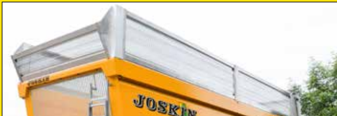
Grated "silage" type extension
