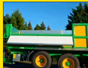
Folding side with hydraulic control
