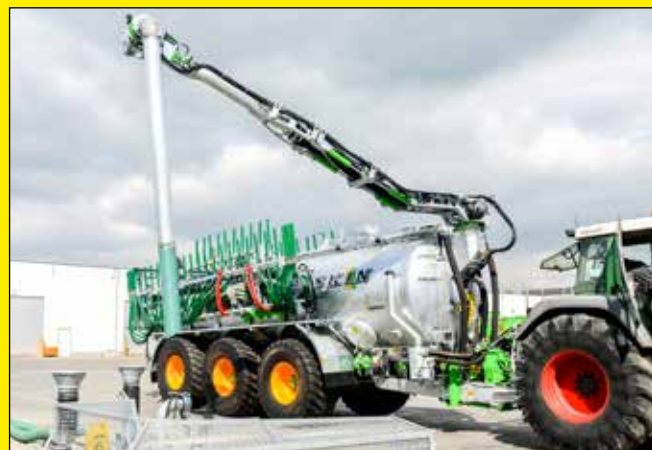
New dorsal boom with pivoting point at the front
