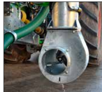
Submerged turbo on articulated arm
