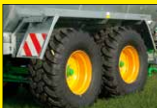
Mudguards on double axle WITH-OUT wheel recessing
