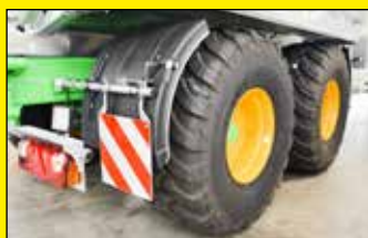
Mudguards on Vacu-CARGO with independent flaps
