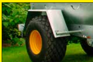
Mudguards on single axle WITH-OUT wheel recessing
