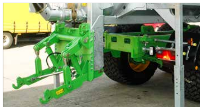
CARGO Low-lift linkage on VACU-CARGO
