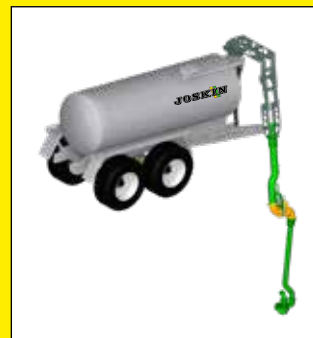
Front boom with submerged turbo
