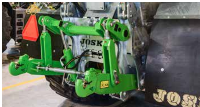
Integrated Lift linkage in the tank on VOLUMETRA
