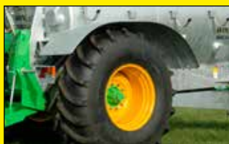
Mudguards on single axle WITH wheel recessing
