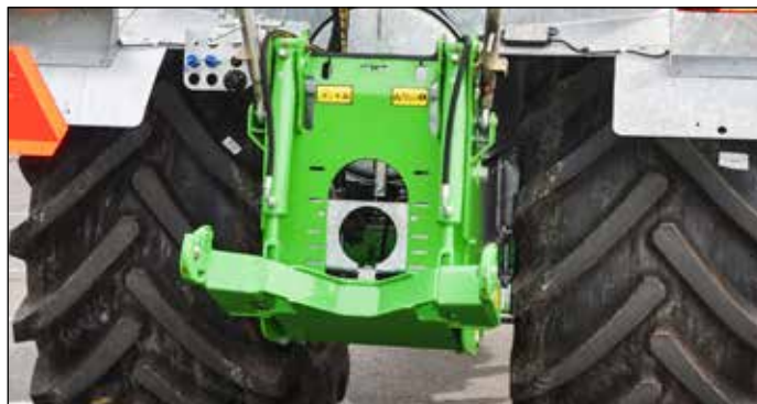
L600 linkage on COBRA (fastened by 4 tapered shafts to make it a solid construction)
