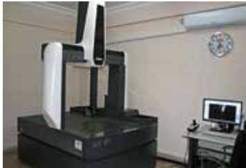
3 Coordinate Measuring Machine - Wenzel LH 87 - X = 800 - Y = 1000 - Z = 700 mm
