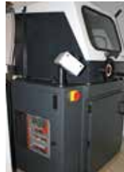
Cutting Machine - IMPRO Procult - Metallographic Cutting Machine
