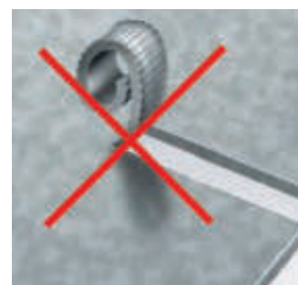
Notching without chip breaking
