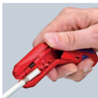
Stripping of a coax cable
