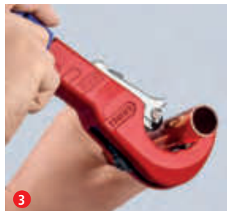
3 Tighten and cut with a swift twist and then readjust using the ergonomic blue feeding barrel...
