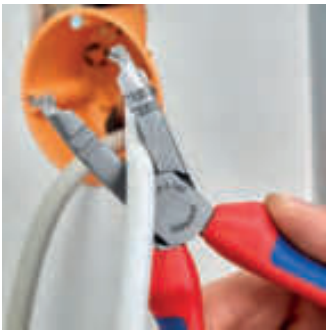
Cutting cable up to Ø 13 mm
