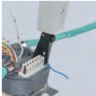
Inserts and cuts cables in one operation
