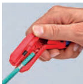
Stripping of a data cable
