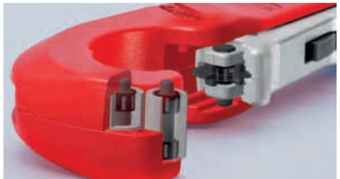
High-quality needle bearings enable the cutting wheel and the four guide rollers to operate virtually without any friction during the cutting – cuts stainless steel pipes with particular ease
