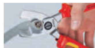
Final cut: after cutting the sheath in the front profile the conductors in the rear part are cut. Initial cut in the front profile, final cut in the rear profile – to keep it as easy as possible.
