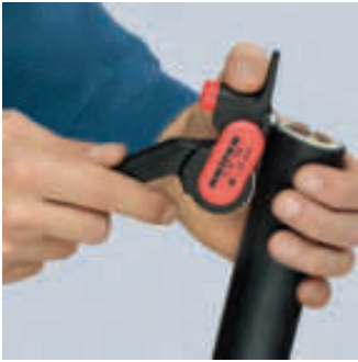
Setting the tool for longitudinal cut
