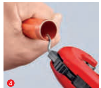
4 and you're done! If necessary, have the edge smoothed out using the fold-out deburring tool – with surprisingly little effort
