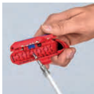
Stripping of a coax cable
