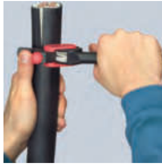
Turning the tool for circumferential cut
