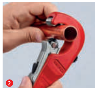
2 Push the cutting wheel against the pipe with the QuickLock single hand quick adjustment: fastest adjustment to different pipe diameters
