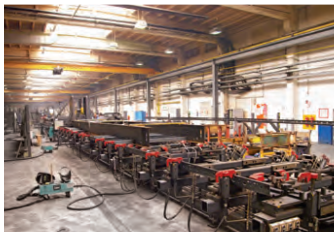
Welding jigs help to achieve extremely precise welding.
