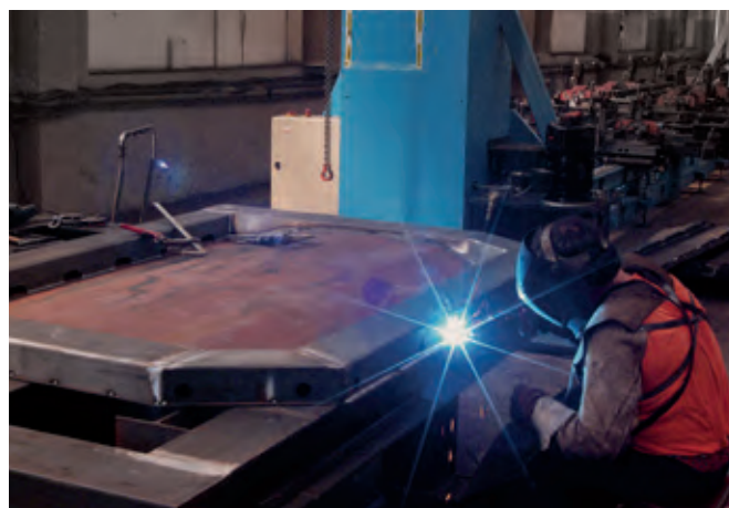
Here we create the back wall of the Kögel Tipper Trailer.
