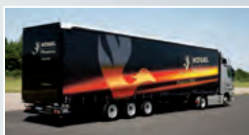
Lightweight study Phoenixx: Floor frame, throat, front wall and rear portal made of carbon fibre
