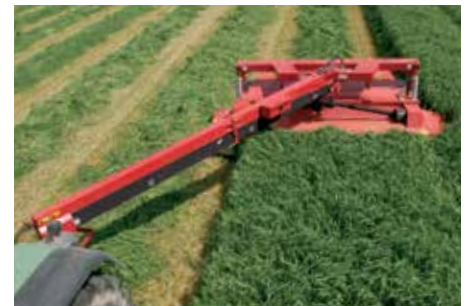
The Flex machines are equipped with a long, strong central drawbar.
