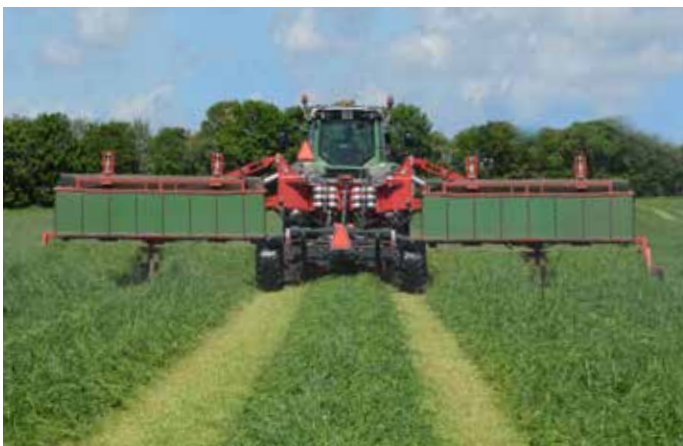
GXT 13005 P - working width 12.3 m.
