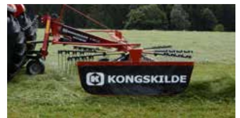
Rake R+ 365 with adjustable swath curtain.
