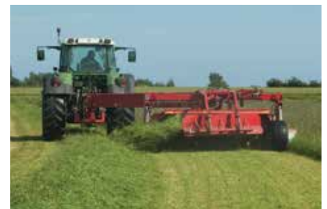
The GMT L /Flex mowers can be fitted with the equipment "Collector" for double swathing. With this equipment you can lay double swaths for the following machinery and thereby optimise the machine chain.
