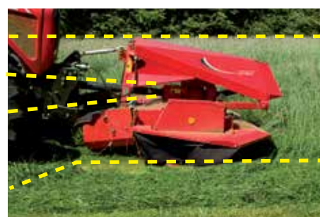
The cutter bar tips back and forth so that it remains parallel to the ground.
