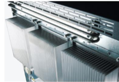
The passive heat exchange system, with separate air circulation in the inner and outer zones of the controller, allows low-maintenance operation even in dusty environments. Entirely without filter mats.
