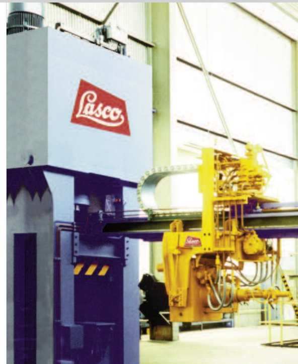
AR 160 stretching press for the production of pre-forms for truck axles.
