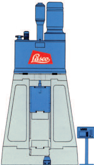
An old belt lift hammer with 30 kJ of blow energy converted to hydraulic drive.
