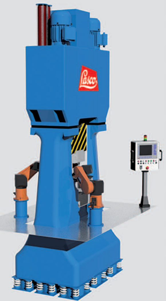
A fully automated die forging hammer from LASCO with synchronized forging robots.
