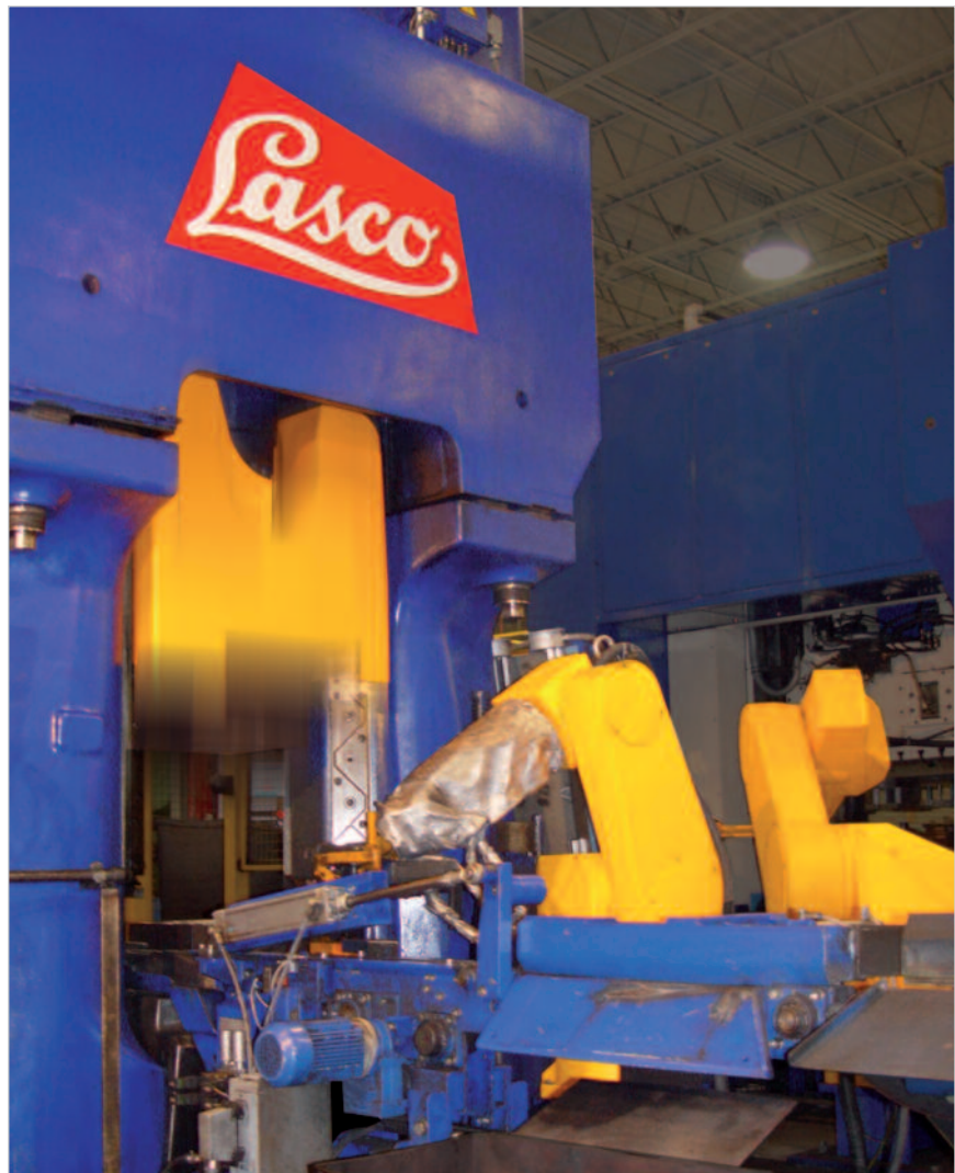
A fully automatic forging line for the manufacture of hand tools.
