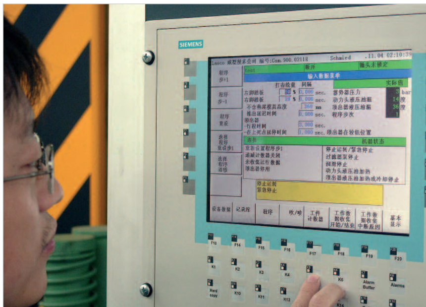
LASCO designs the operator menus and screen forms individually according to the customer's demand, in this case located in China.
