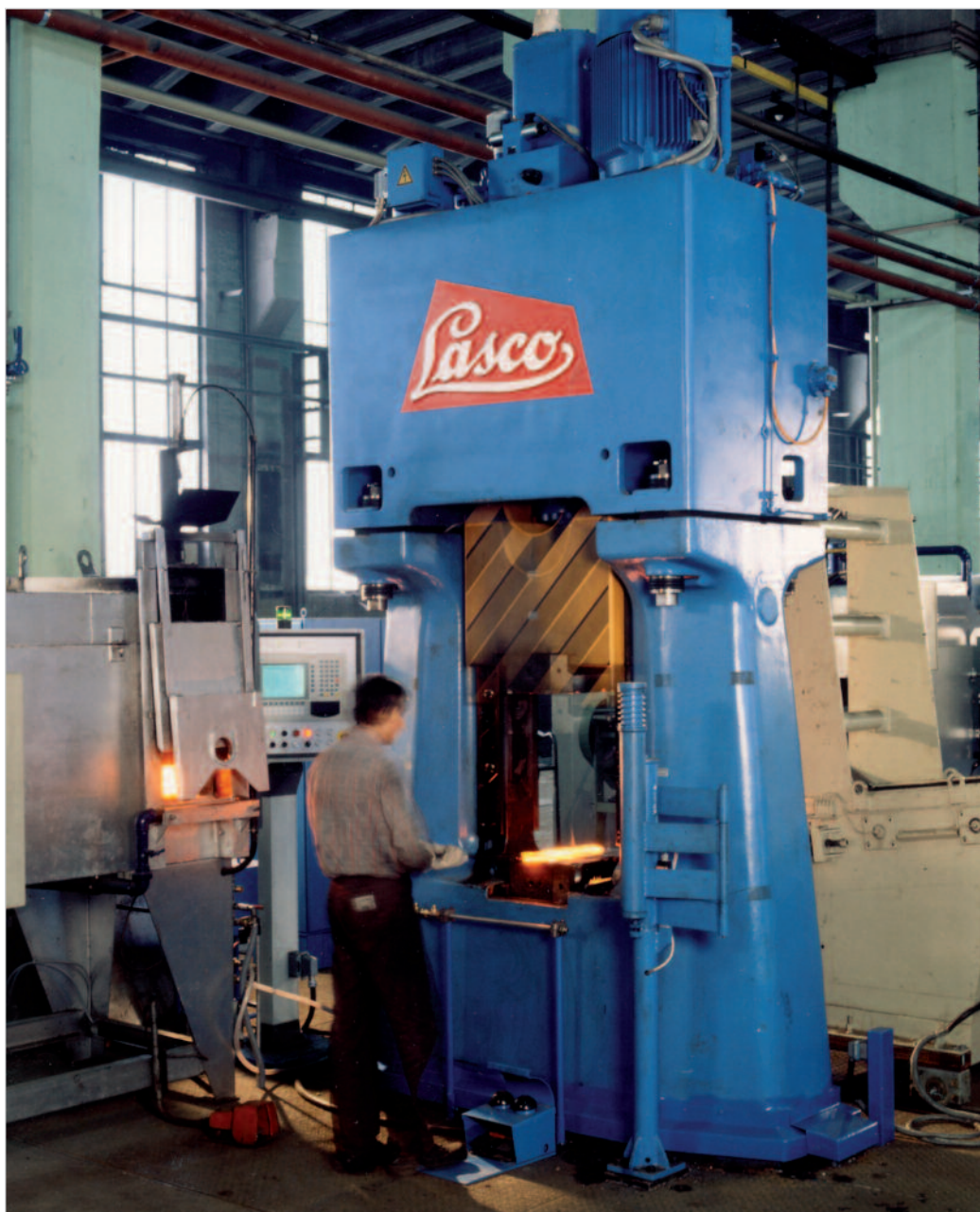
LASCO HO-U 250, 25 kJ blow energy, programmable control.
