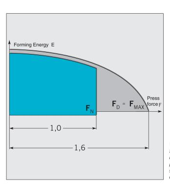
With their high forming force at low power requirement, SPP screw presses are particularly suited to coining and calibrating work.
