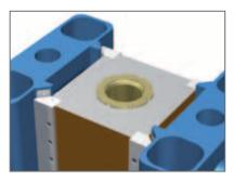
Sectional view of the guiding system for the press ram (SPR 2500).
