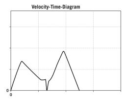
The three velocity-time-diagrams above show the course of the ram at 100, 50 and 10% energy set. The ram is accelerated at maximum possible speed and generatively decelerated at a velocity equivalent to the preset energy. After the forming process and the backlash, the ram is electronically intercepted, accelerated and again generatively decelerated, so that the ram exactly positions in the upper dead center.
