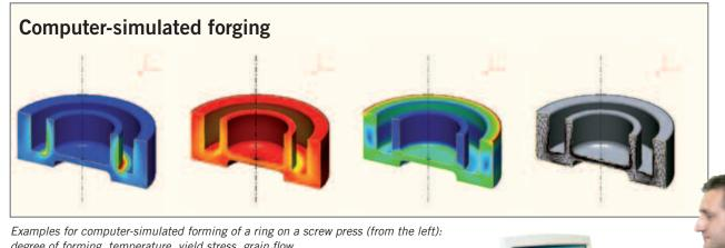
degree of forming, temperature, yield stress, grain flow.
