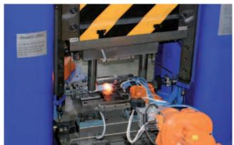
Fabrication of knife blanks on an SPP 400.
