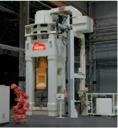
The automated LASCO SPR 1250 screw press working in the facility of an automotive supplier in the USA.
