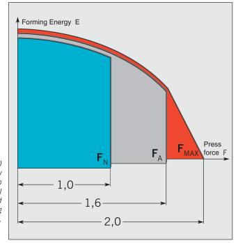
The force of pressure (red) generated by an SPR screw press can be a maximum of twice the nominal force. Machine overload is prevented by a slipping clutch on the flywheel.
