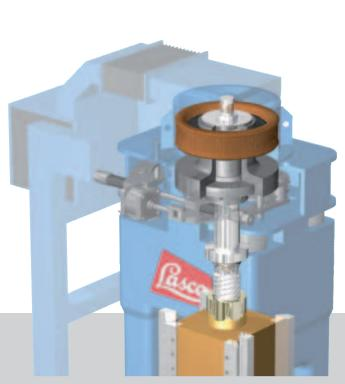
Schematic of the basic design of an SPP series drive.
