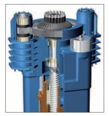
Symmetrically configured three-phase asynchronous motors on the flywheel of a screw press (SPR 2500).
