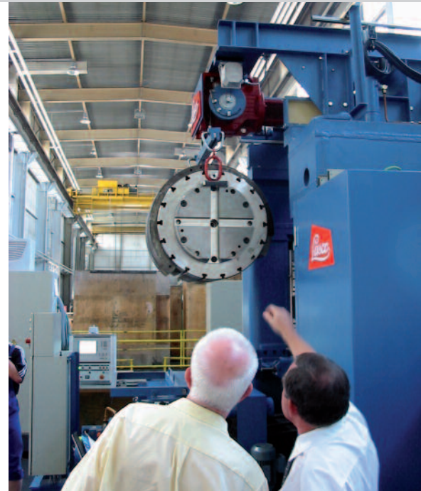
Roller change manipulator. A roller is changed in less than five minutes.
