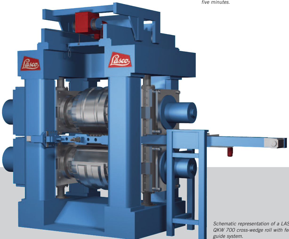
Roller change manipulator. A roller is changed in less than five minutes.
