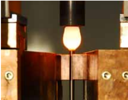
Upsetting on EH (above) and EV (below)
