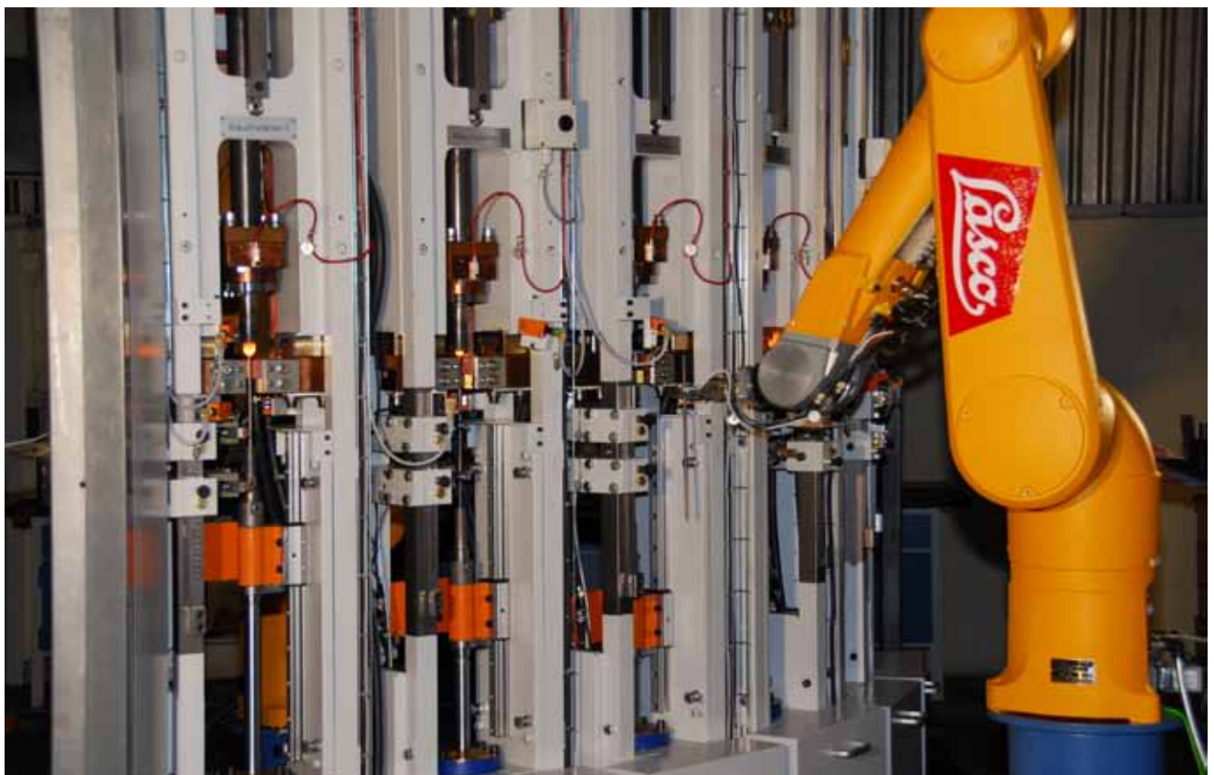
Electro-upsetting line EV 16 with 6 upsetting units
