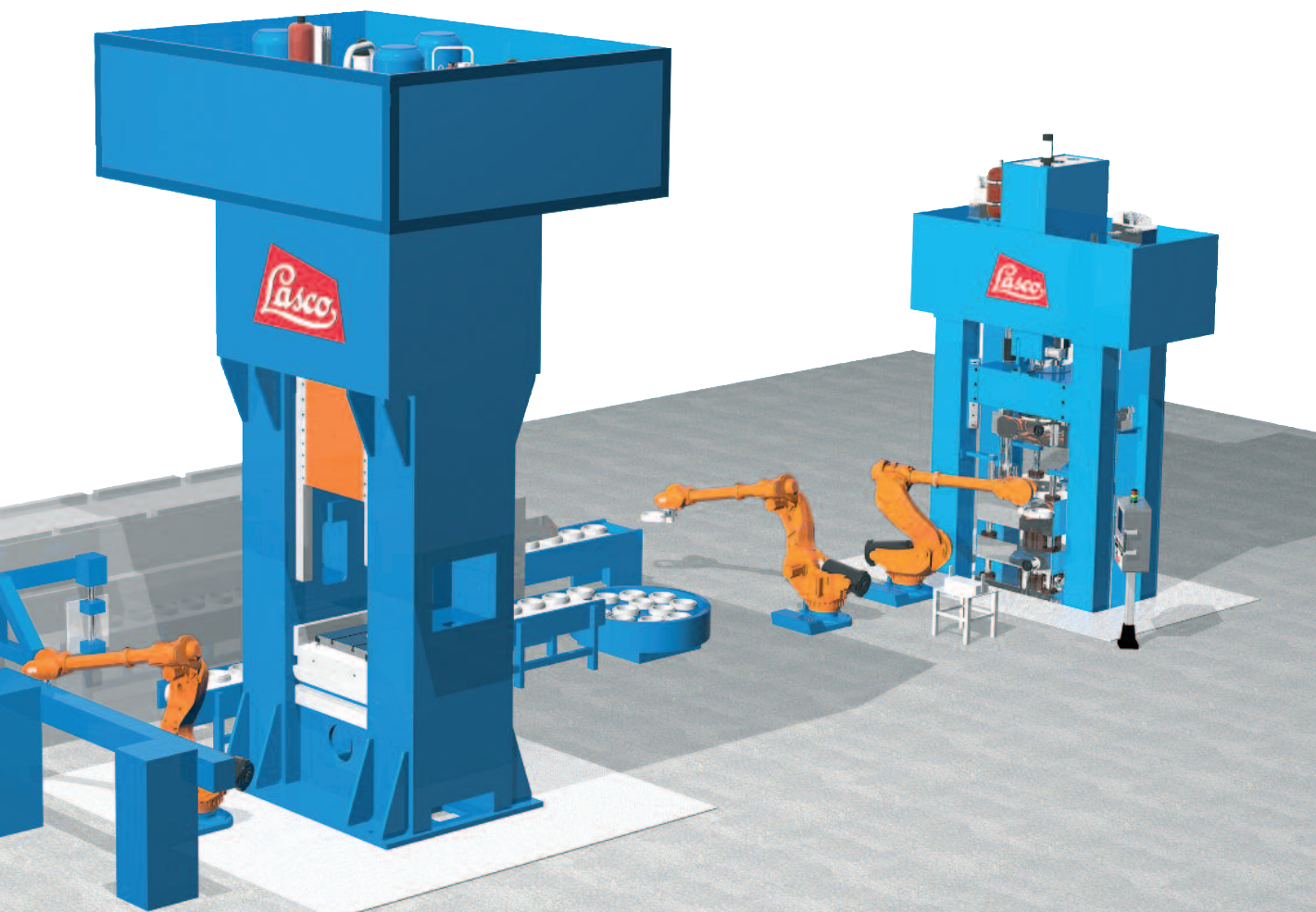
Schematic of two inter-linked LASCO units VPE 500 and MPP 400 with automation devices.
