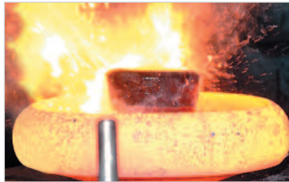
A billet is pre-formed for a ring, on a VPE 800.
