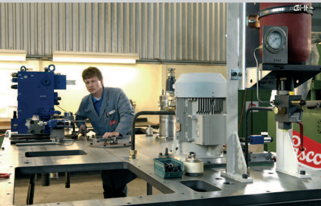
LASCO employees are installing the hydraulic drive of a VPE.
