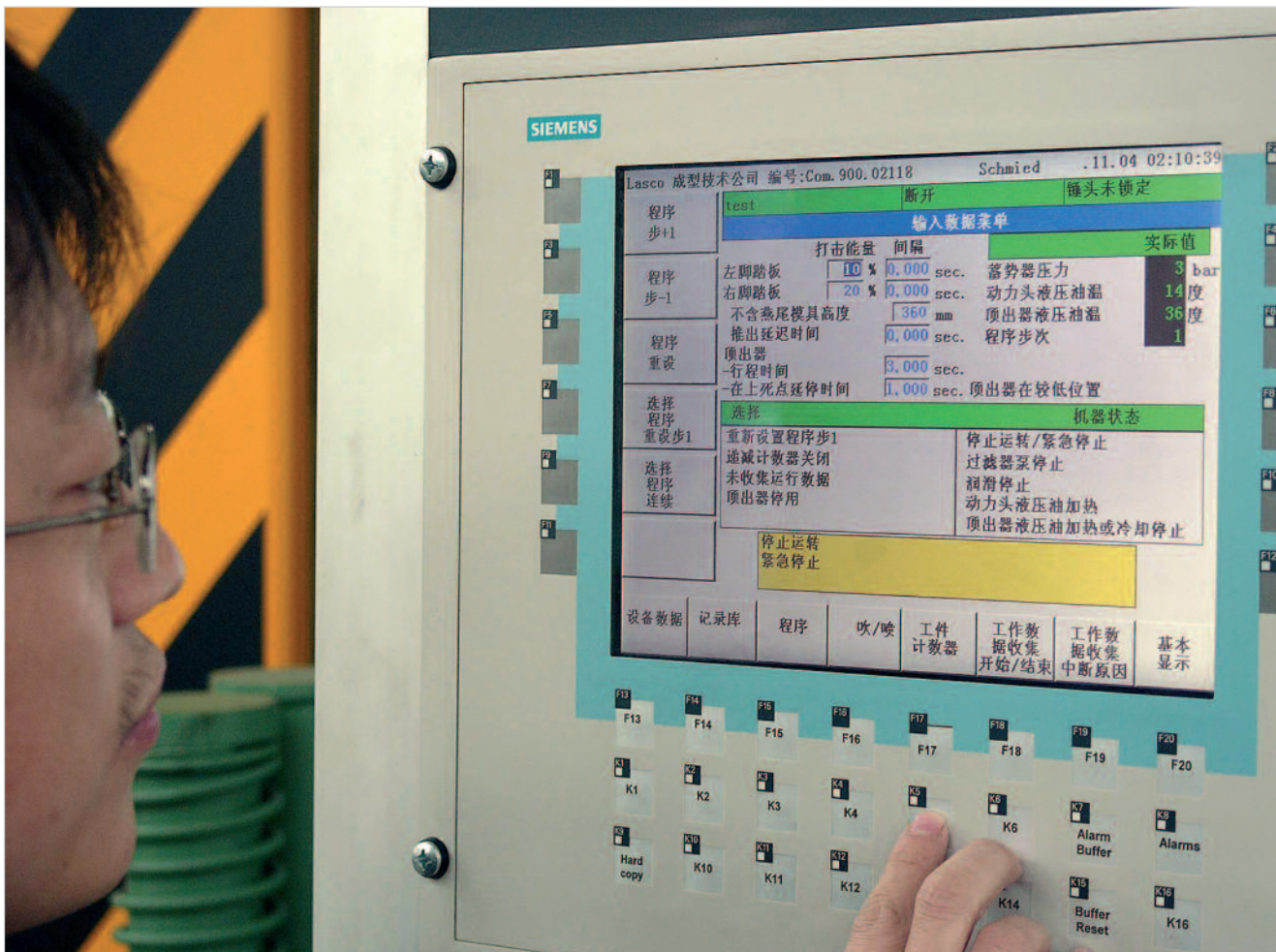
LASCO designs the operator menus and screen forms of a control system individually according to the customer's demand, in this case, located in China.
