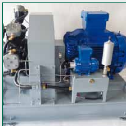
LW1300 EG with additional oil lubrication circuit
