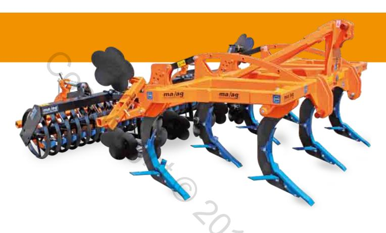
Ideal for minimum working (15-25 cm) and deep working (until 40 cm), it's a real alternative to the traditional tillage.
