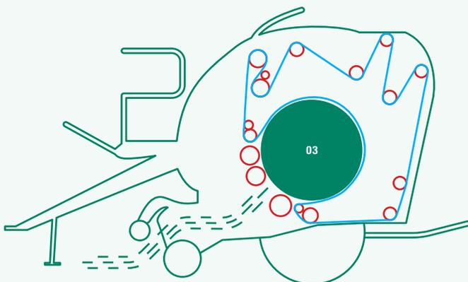
04 Just like the core of the bale, the outer layers are compressed at the same consistent pressure using both springs and hydraulics until the set bale density and size is reached.
