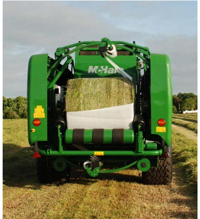
03 As the bale is forming inside the chamber, the hydraulics take over the tensioning of the belt(s) from the four large springs. Two hydraulic rams control the tension on the chamber belt(s) as the bale forms inside the chamber.
