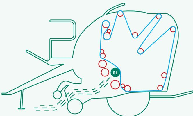
**02** This is done by **four heavy-duty springs** that pressurise the crop at the start of the baling process. The tension placed on the crop by these large springs allows for the perfect start to the bale. The spring tension on the belts ensures easy bale formation and a properly formed core.
