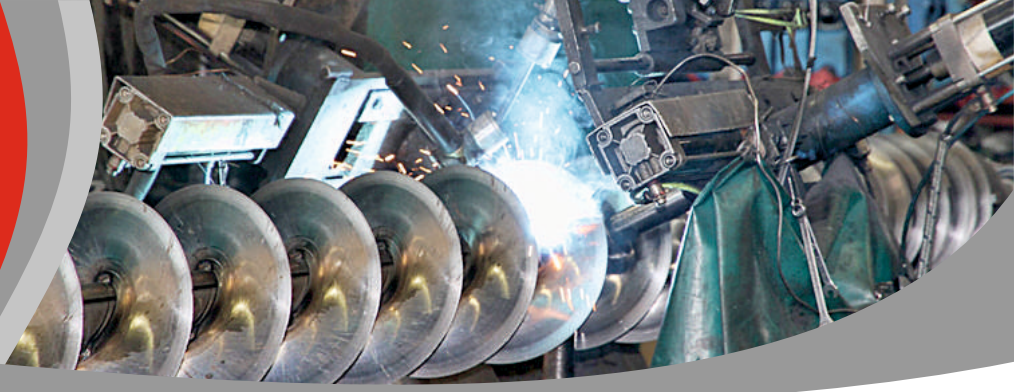
Boruya Kaynaklı Helezon Krom ve Siyah Carbon Steel Or Stainless Steel Screw Flight Welded On Shaft / Pipe
