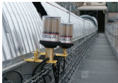
Mineral industry: lubrication of conveyor belt bearings.
