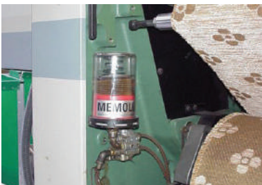
Textile industry: Picanol weaving loom bearings.
