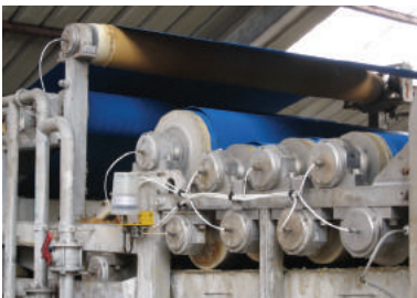
Food industry: lubrication of press ball bearings.
