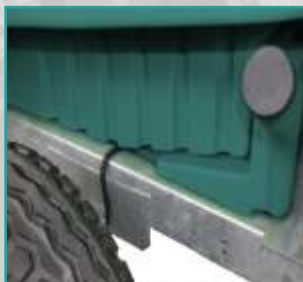
Serbatoio lava circuito Circuit washing tank
