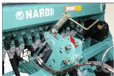
Erpice copriseme e pedana Seed covering harrow with foot board- Herse couvre-graines et passerelle Grada cubresemilla y plataforma
