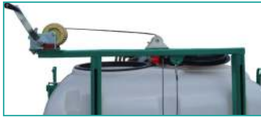
Verricello sollevatore della barra Winch lifting the booms *Standard per barre autolivellanti *Standard feature for self-leveling booms
