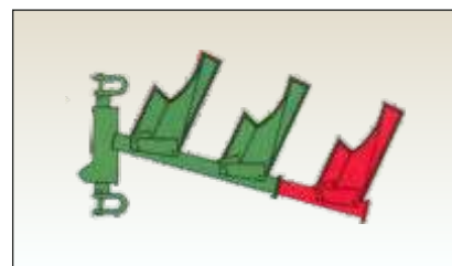
Bivomere trasformabile a trivomere Two furrow plough transf. into three furrow plough Bisoc transformable en trisoc
