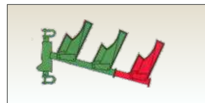
Bivomere trasformabile a trivomere Two furrow plough transf. Into three furrow plough Bisoc transformable en trisoc
