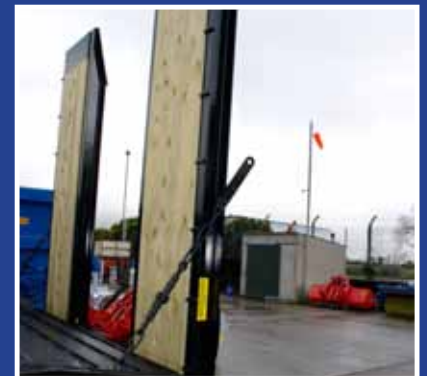
Softwood Sheeted Ramps
