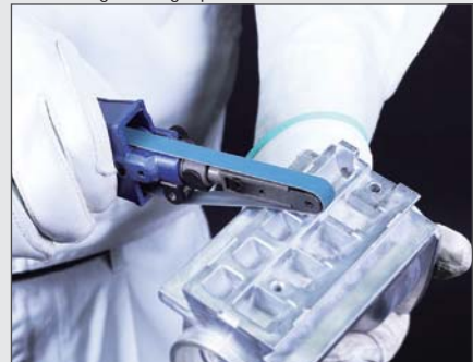
Chamfering of straight parts.
