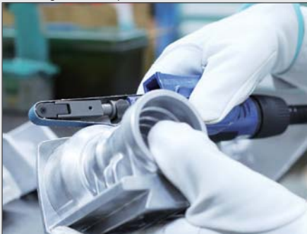
Deburring of die cast parts.
