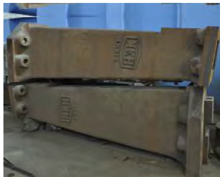
Raw Casting of Columns
