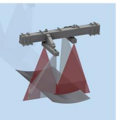
In light-section measurements, a laser arranged at 90° above the strip projects a laser line onto the strip surface. A camera installed at an inclined angle above the strip in a sensing unit captures this projected line (Picture: nokra)
