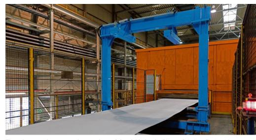
The exit gauge documents the crossbow of the pickled strip (Picture: Salzgitter Flachstahl)
