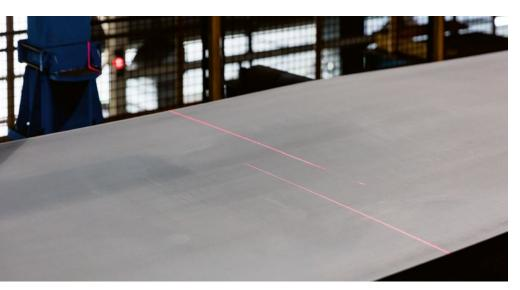
The two laser lines projected across the running strip are offset in order to avoid cross-talk between the two channels (Picture: Salzgitter Flachstahl)
