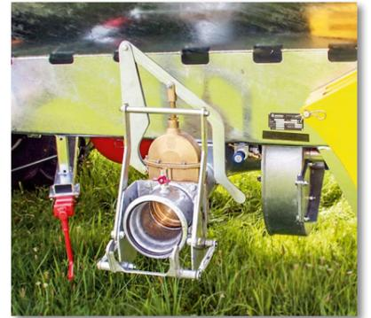
Power Fill 6"/" Rotor 450 mm Ø
