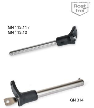
The new locking pin also offers high security with regard to its load carrying capacity. Ganter determined the double shearing resistance in accordance with DIN 50141. In the test setup, the pin connects an element to another that encompasses it. The force that results in a break in both shear planes is then measured. For a locking pin with 10 mm diameter, the shearing resistance is 46 kN, while a 20 mm pin can withstand 227 kN.
