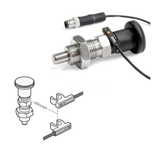
Thanks to the standard connection dimensions, the plunger can easily be used as a replacement for typical indexing plungers. All variants consist of Stainless Steel because this material only minimally shields the integrated magnet, thereby avoiding interference with the functioning of the sensor.
