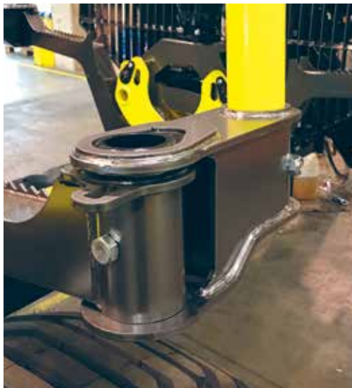
Loading area widening for forwarder type bolsters
