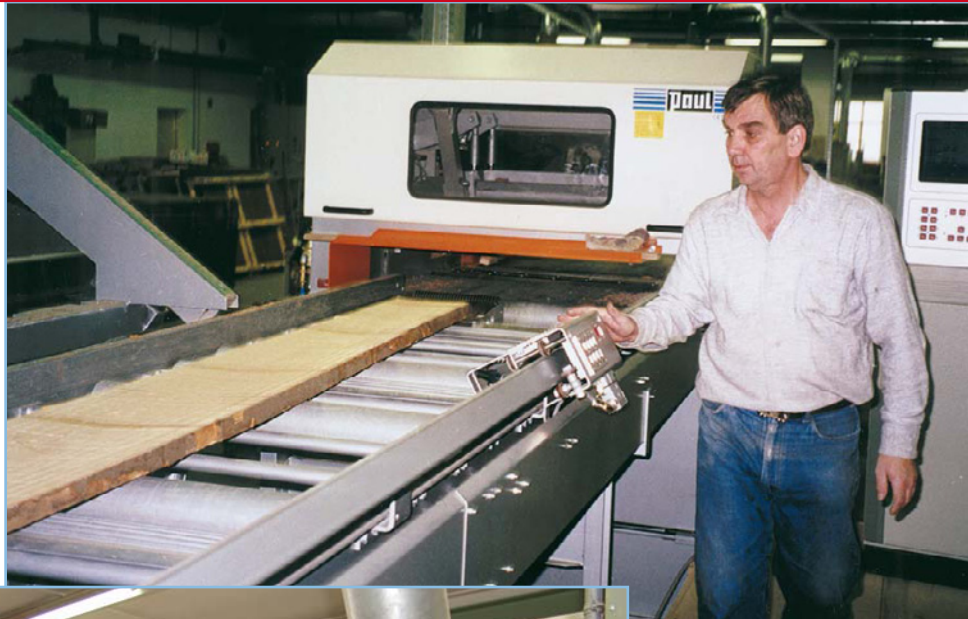
Fig. 6 Movable measuring carriage for the non-contact cutting point and defect marking
