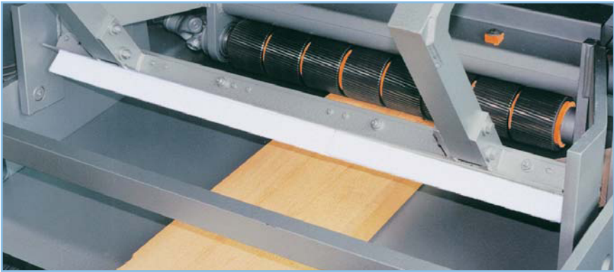
Fig. 3 Inside view of a model 18GE: Segmented top rollers, tilting sweeper
