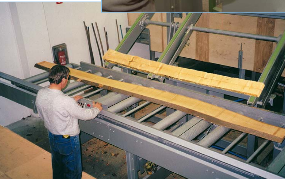
Fig. 8 Non-contact grading by means of a laser and function keys
