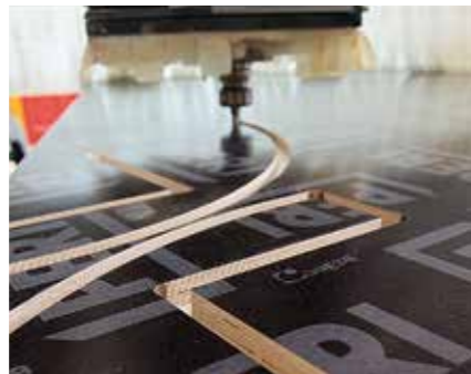
Individually tailored plywood sheets are accurately produced using modern CNC equipment.
