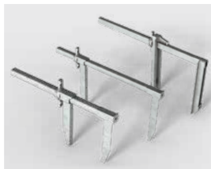
With PERI Wall Clamps, small beams and up to 90 cm wide strip foundations can be realized. The Quick Jack Nut allows friction-locked fine adjustment.
