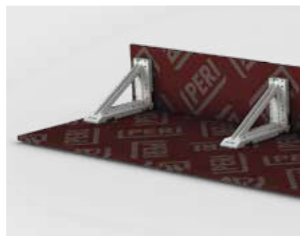
With the plastic PERI Slab Stopend Angle, beams up to 60 cm high and slab edge stopends up to 40 cm can be formed. The Slab Stopend Angle is simply nailed to the wooden girders or formwork sheets.
