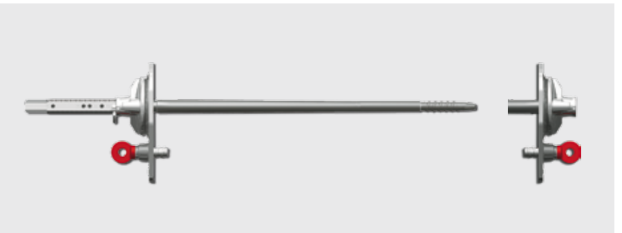
The wall thickness can be easily adjusted on the anchor by means of a cotter pin. The usual wall thicknesses are indicated through markings on the tie rod.
