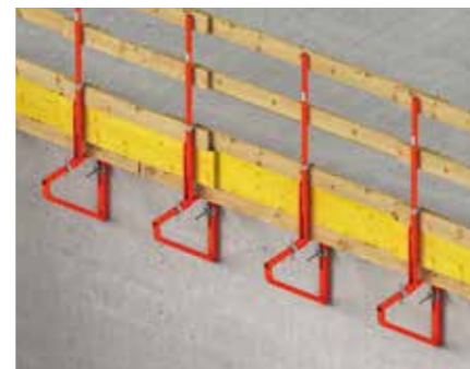
The Formwork Bracket-2 is used for forming cantilevers of up to 45 cm with slab thicknesses reaching 30 cm.
