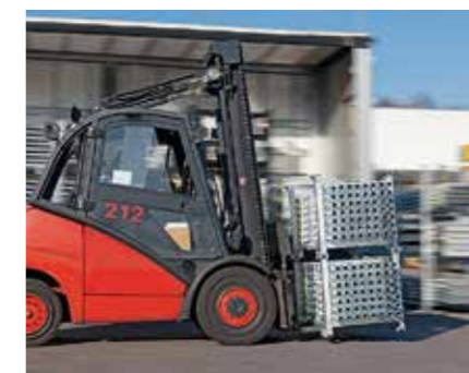
For fast and safe transportation with the forklift, PERI pallets are placed on top of each other.
