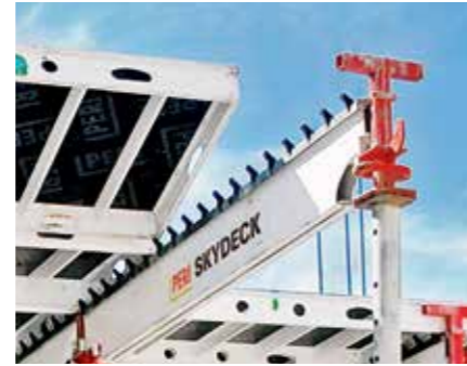
The size of the panel dictates the respective prop position, measuring is not required. The outward projecting teeth on the longitudinal beams secure the panel against moving out of position.
