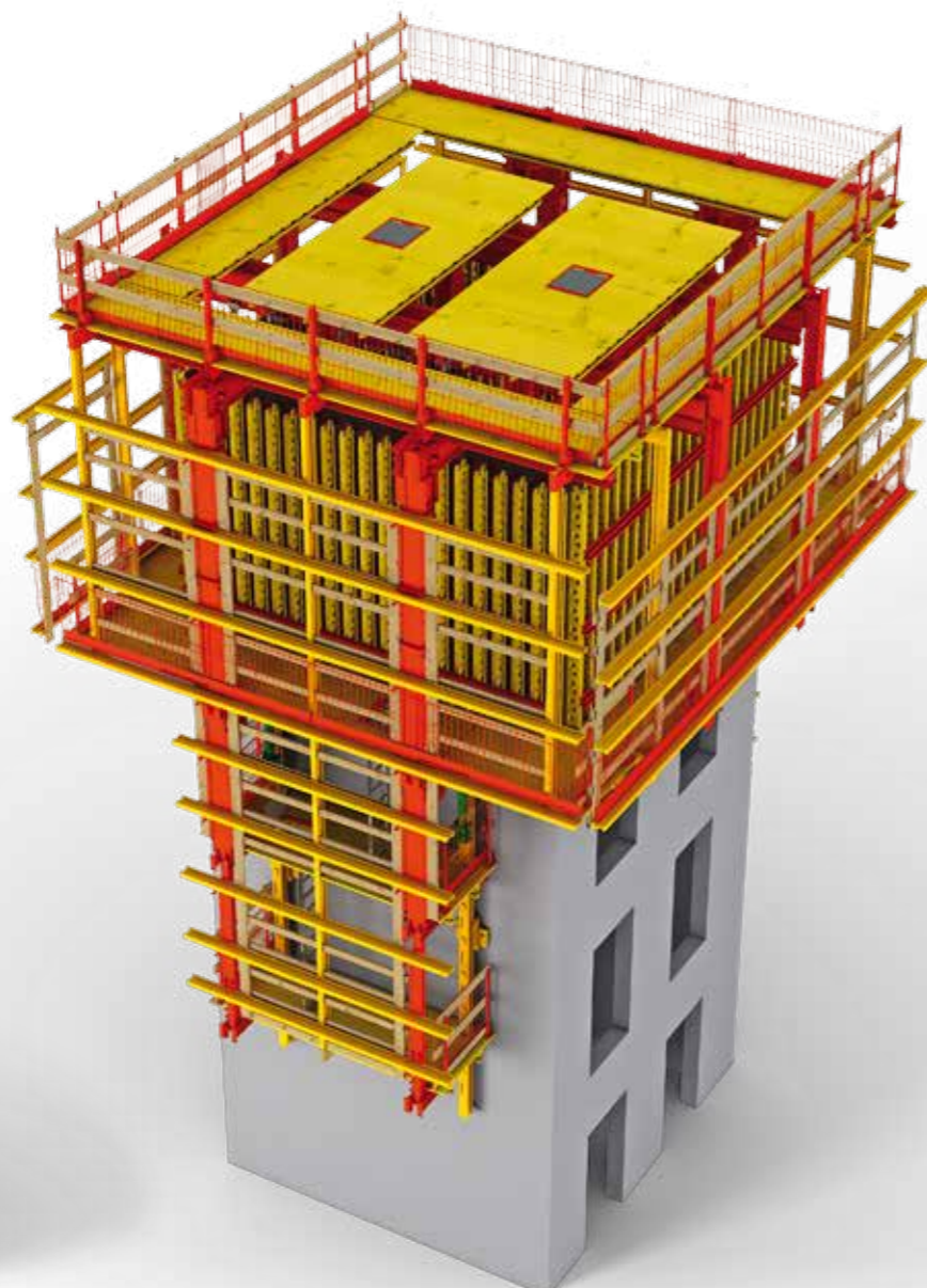
ACS P – the solution for advancing cores of high-rise buildings and tower-like structures – combined with ACS G. Both formwork sides are movably attached to the cantilevered platform beams.
