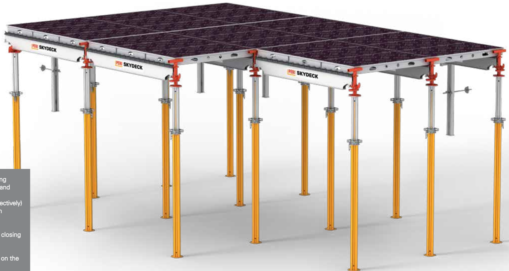
The size of the panel dictates the respective prop position, measuring is not required. The outward projecting teeth on the longitudinal beams secure the panel against moving out of position.
