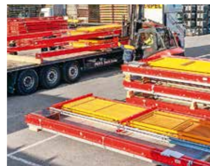
The platforms can be stacked pre-assembled and space-savily transported. The guardrails are simply inserted on the construction site.
