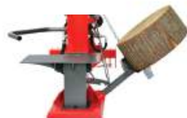
Additional lifting device for short logs-optional
