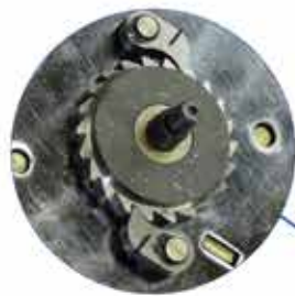
Safety brake with two stainless steel pawls
