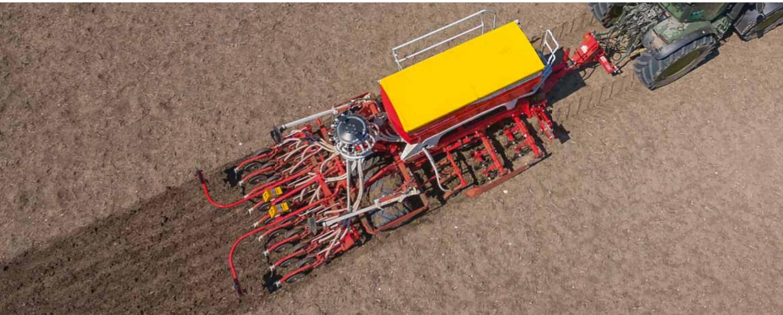
The low draft WAVE DISC with a diameter of 510 mm is designed especially for low disturbance drilling. The soil around the WAVE DISC is not moved to the side, but is loosened in strips, thus preventing smearing at seed slot level. Row spacings of 12.5 or 16.7 cm are available. A row spacing of 16.7 cm is recommended for regions with extremely heavy, wet and sticky soil conditions. The WAVE DISC is available for all TERRASEM mulch seed drills.
