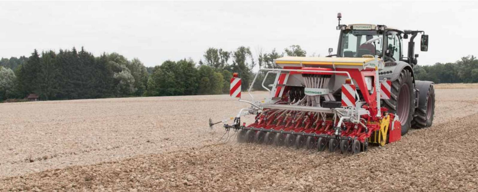
The unique AEROSEM seed drill concept from PÖTTINGER unites the drilling of cereals and maize. Precision universal metering and perfect coulter systems guarantee exact placement of the seed.
