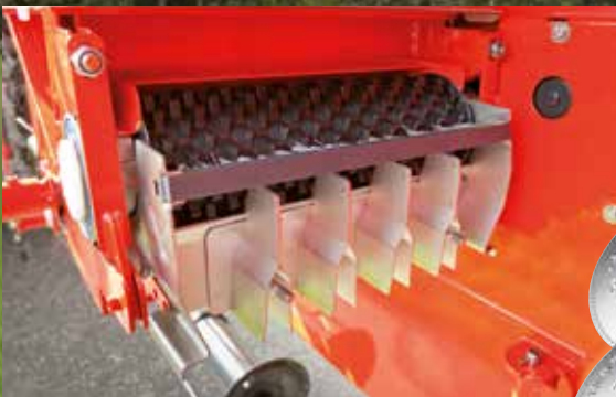
A separate metering unit for each boom section
