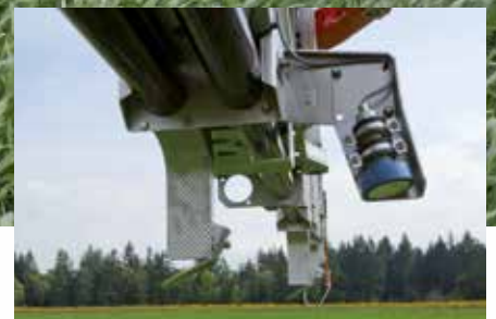
Distance control: Ultrasonic sensor
