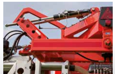
Distance control: Automatic boom guidance
