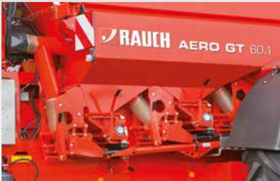
Three separately adjustable metering units on each side
