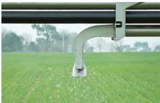
Vortex chamber manifold
