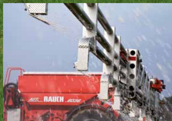
A separate metering unit for each boom section
