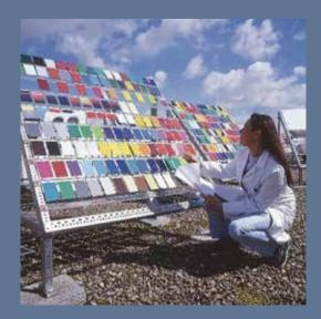
Solar Shield Technology (SST) is featured in all of our exterior-grade laminates to significantly reduce thermal heating and help ensure that profiles retain their dimensional stability even when exposed to strong sunlight.
