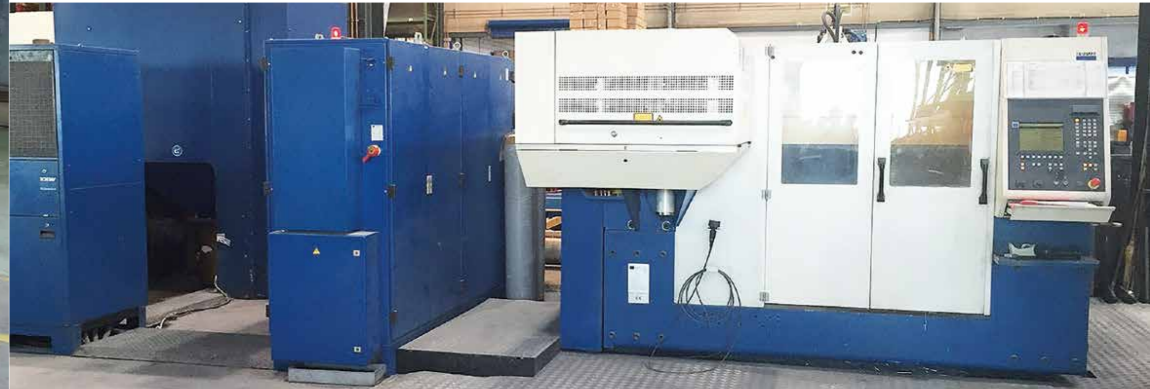
SORALUCE TR 35 Flatbed milling machine ≤ 3.500 mm x 1.250 mm x 1.500 mm Single measures up to 10 tons
